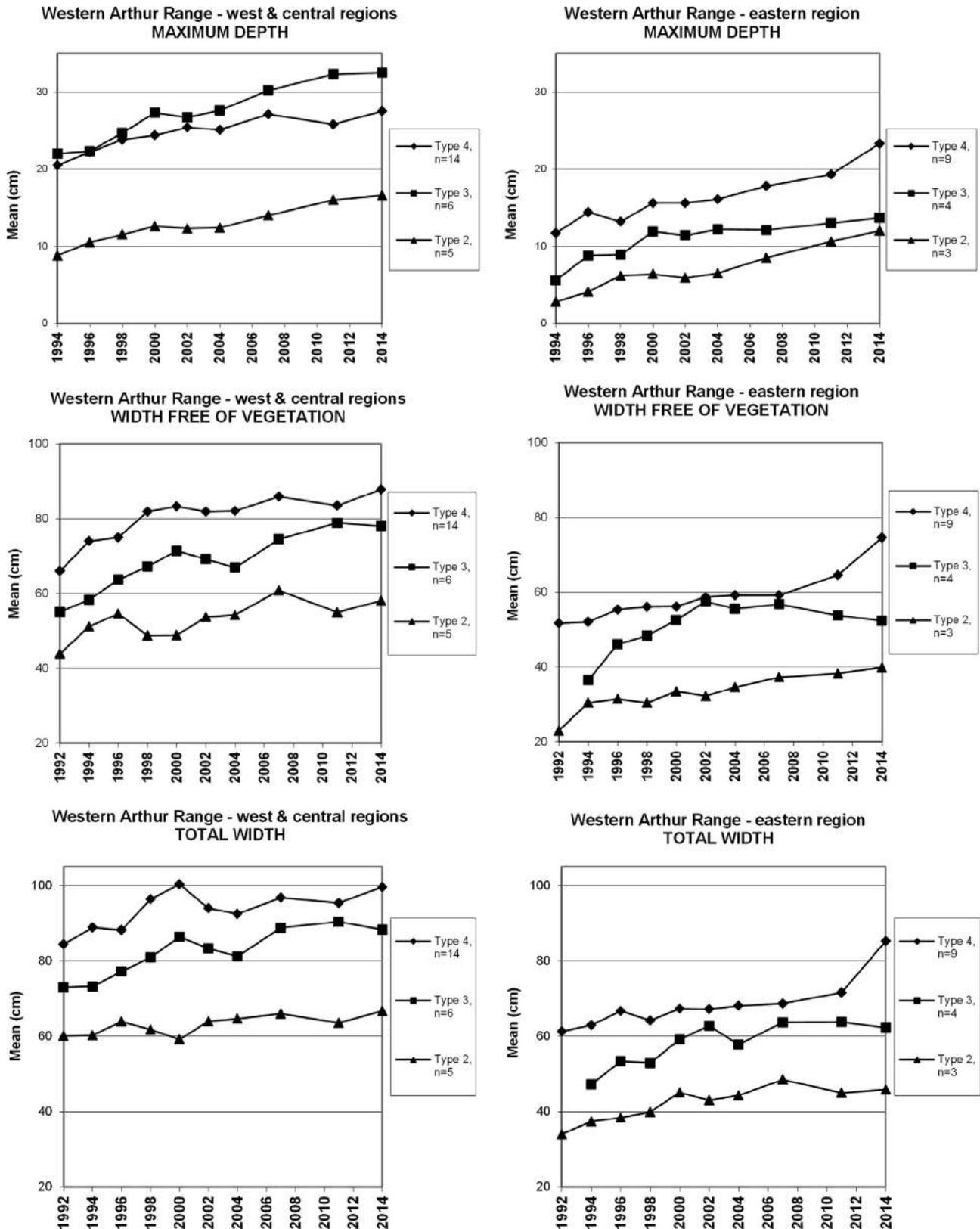
Fig. 2. Changes in impact parameters at clustered-transect monitoring locations in the Western Arthur Range. Types are a method of describing a site's susceptibility to erosion or widening; sites were classified by Type based on environmental and siting factors (see Section 4.2).
