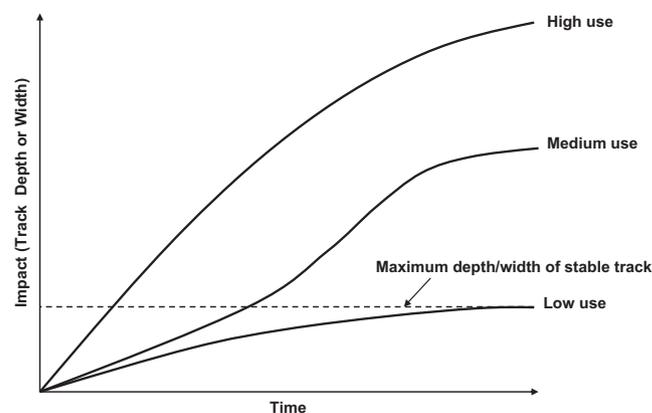
Fig. 9. Inferred impact/time curves for different use levels.
